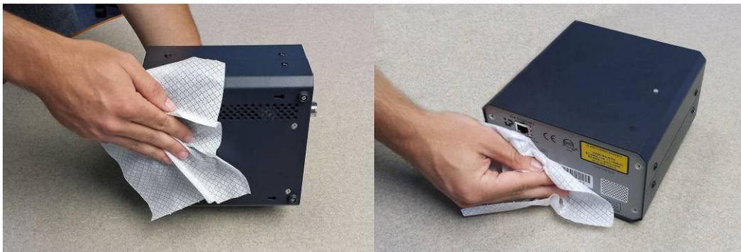
Figure 3- Cleaning the Exhaust Ports
