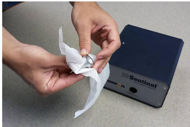
**Figure 5- Cleaning the Nozzle**
