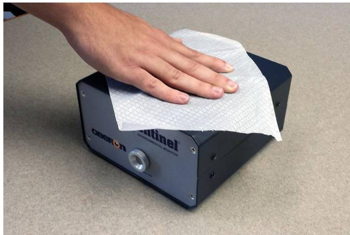
Figure 2- Wiping Down the IC Sentinel
